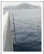
A pole installed to sustain only the sensor arm. The length is 2 m and the distance between the supports is about 1.8 m
