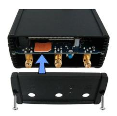
In order to insert the SIM in the router it is necessary to remove the router from the control box with a small cross screwdriver (two small screws at the side of the router), and open the router as indicated in the figure.
