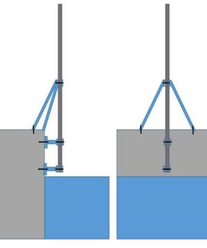
In case the lower support can be part of the day under water, it is necessary to wait the low tide in order to perform the installation. This is more a problem for Atlantic Ocean locations where the tide excursion is much larger.
