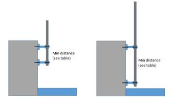
Once identified the right vertical wall that allows the fixing of the supports with their minimum distance, it is usually necessary to involve specialized personnel (Fire Fighters or Mountain specialists) that will work appended outside the vertical wall to drill and fix the supports.
