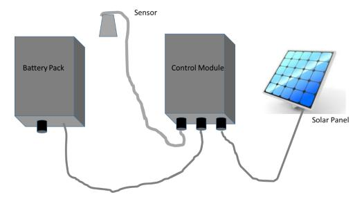
Please make sure not to connect wrongly the 3 connectors as it may damage the sensor.
